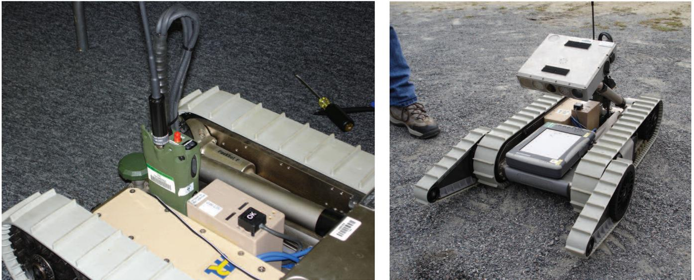
**Figure 1.** WSRT integration onto PackBot® (left) with tablet PC for data collection (right).
