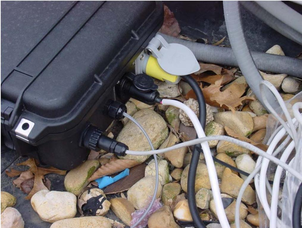
Figure 3. Bulkhead connectors on exterior of conversion box.
